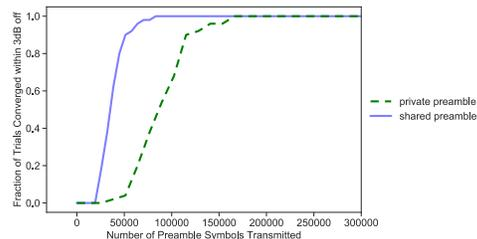
Fig. 4: Convergence of 50 Neural-vs-Clone trials to be within 3 dB (at testing SNR 8.4 dB) using the EPP and ESP protocols at 2 bits per symbol and training SNR 8.4 dB. EPP takes more symbols to converge.
