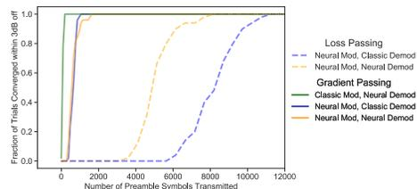
Fig. 3: Convergence of 50 GP and LP trials at 2 bits per symbol to be within 3 dB (at testing SNR 8.4 dB) at 8.4 dB training SNR. LP requires more symbols than GP to converge.
