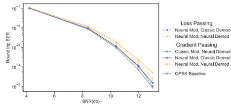
Fig. 2: Round-trip median BER curves for GP and LP protocols at 2 bits per symbol and 8.4 dB training SNR. Permutations of neural and classic modulator and demodulator models are tested in order to show individual learning components independently. (a) is the full curve at all test SNRs and (b) is zoomed in on the upper end of the testing SNRs. All of the loss and gradient passing settings show close to baseline performance.
