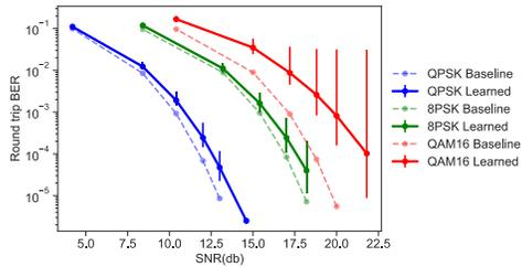
Fig. 6: Round-trip median BER curves for Neural-vs-Clone learning QPSK, 8PSK, and 16QAM under the EPP protocol at training SNRs corresponding to 1% BER. Alongside the BER curves of the learned modulation and demodulation schemes is the baseline. In all cases, modulation constellations are normalized to constrain the average signal power. The learned 16QAM agents perform worse relative to the baseline than QPSK and 8PSK agents.
