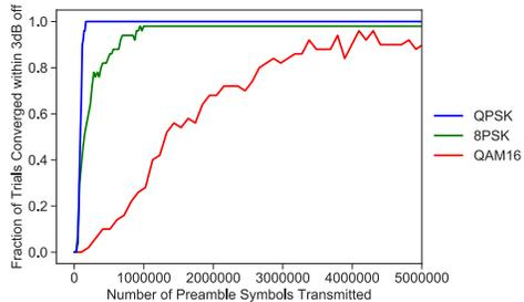
Fig. 7: Convergence of 50 trials to be within 3 dB (at testing SNR corresponding to 1% BER) of the corresponding baseline for EPP trials of Neural-vs-Clone at training SNR corresponding to 1% BER for increasing modulation order. 16QAM, with the highest modulation order 4, takes much longer to converge than QPSK (order 2) and 8PSK (order 3).
