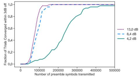
Fig. 8: Convergence of 50 Neural-vs-Clone trials to be within 3 dB (at testing SNR 8.4 dB) at 2 bits per symbol using EPP protocol at training SNRs 13.0, 8.4, and 4.2 dB. Training at higher SNR reduces the number of symbols required for most seeds to converge.
