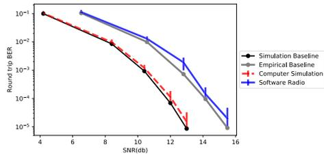
Fig. 9: Round-trip median bit error curves for Neural agent vs clone python simulation and gnradio agent learning QPSK under the EPP protocol at training SNRs corresponding to 1% BER. Alongside the bit error curves of the learned modulation and demodulation schemes is the baseline
