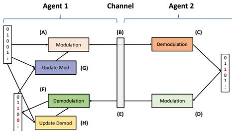
Fig. 1: Visualization of the Echo protocol. (A) Speaker Agent (A1) modulates a bit sequence and (B) sends it across a (AWGN) channel. (C) Echoer Agent (A2) receives the sequence and demodulates it; (D) A2 then modulates the recovered sequence and (E) sends it back over the channel. (F) A1 receives this echoed version of its original sequence and demodulates it. (G, H) Then A1 uses the received echo to update its modulator and demodulator. The agents switch roles and repeat until convergence.
